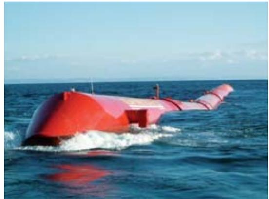
▲ Wave energy devices made by Ocean Power Delivery derive electrical power from the flexing motion at their joints as waves pass underneath. Because they dive into oncoming waves, the Pelamis machines can survive the high seas that accompany intense storms.
